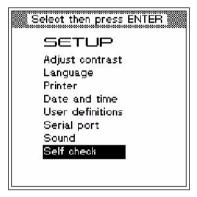
As a rule, the basic settings need only be configured once during initial startup. A powerful capacitor ensures that the settings and the stored test result are preserved when your Willtek 4100 is off.
