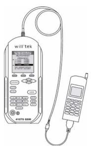
The cable-based connection of the test unit is the ideal choice for precision measurements.
