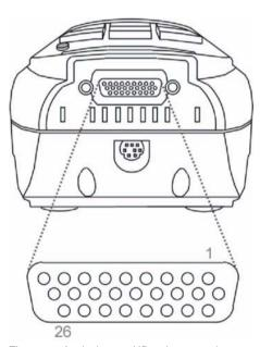
The 4100 includes an HD sub-26 socket to connect to a printer or a PC. An adapter for parallel and serial interface cables is available as an accessory. See the user guide for a description of different applications.
