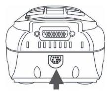
1 Plug the 8-pin connector coming from the power supply unit into the matching socket on your Willtek 4100.
